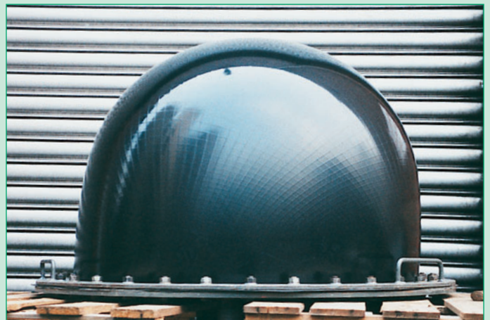
Fig. 8: Burst test of a Carbofol® according to EN 14151
