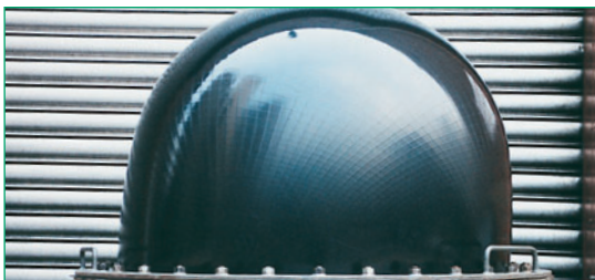
Burst test of a Carbofol® geomembrane according to EN 14151
