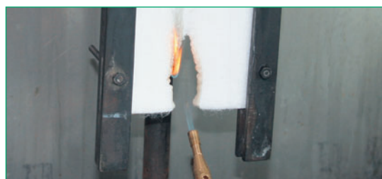
Flame test to determine fire classification E according to ISO 11925-2
