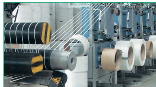
Fig. 4 Stretching process of Secugrid® ribs
